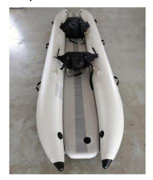
**Step 1:** Remove the tube set from the carrying bag and lay it spread out on a flat surface. Check that the valve plugs are in the filling position.
